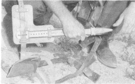
FIGURE 6. Gaff Guard Installed
