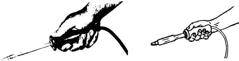
FIGURE 2. Hand Grip Method of Holding Soldering Iron
